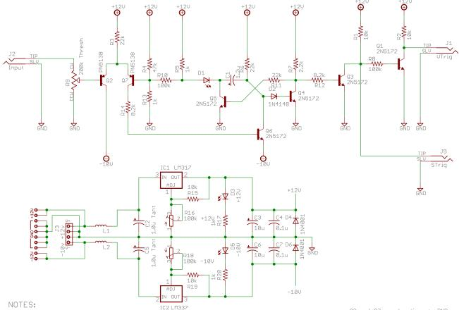
If regulators are not needed/used, do not install the associated components such as C2, R15, R16, R17, and D3 for the LM317, and  $\,$
